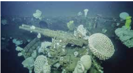
A Bofors 40 mm gun mount remains intact on the port side of Independence. This and other images may be found at www.nautiluslive.org .
