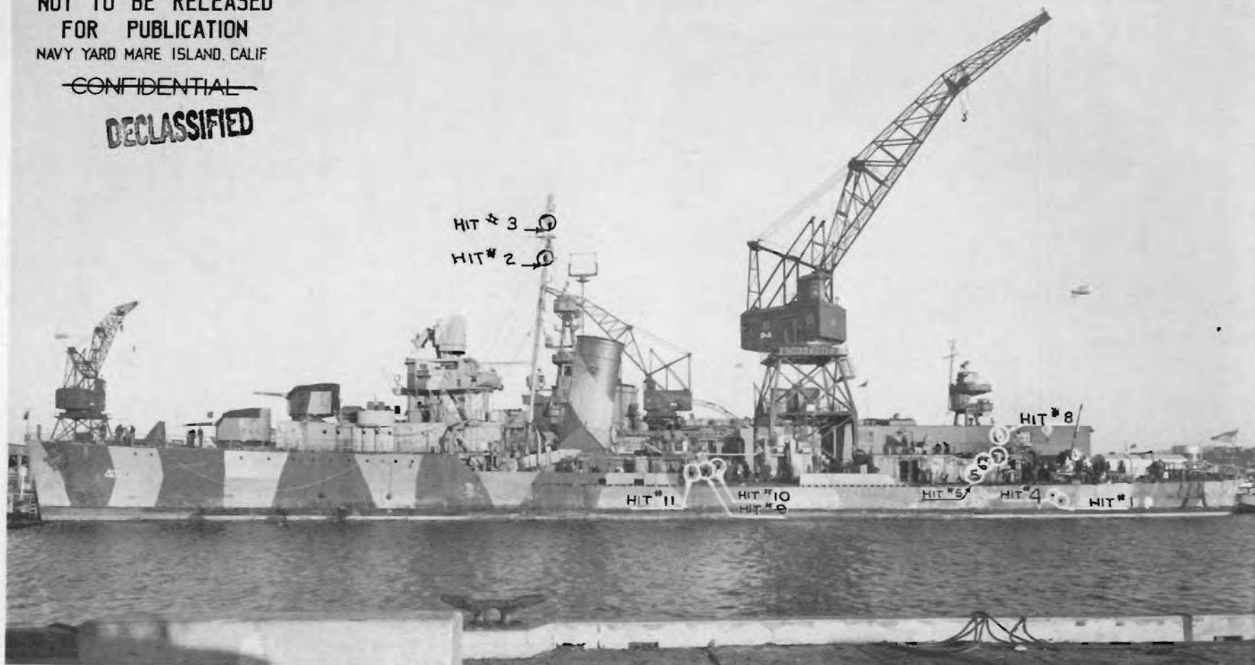
Photo 1: Outboard port profile showing location of projectile hits.
